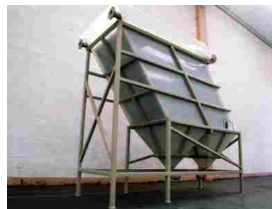
Polypropylene Inclined Plate Clarifier
