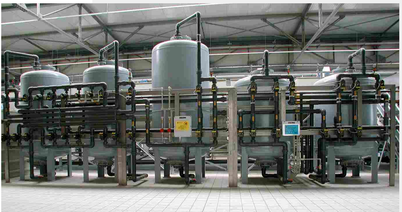
Polishing Selective Ion Exchange System - 20 mc/h
