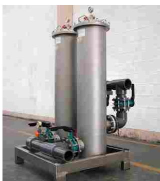
Cartridge filtration on skid
