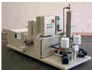
Copper separation and water recycle
