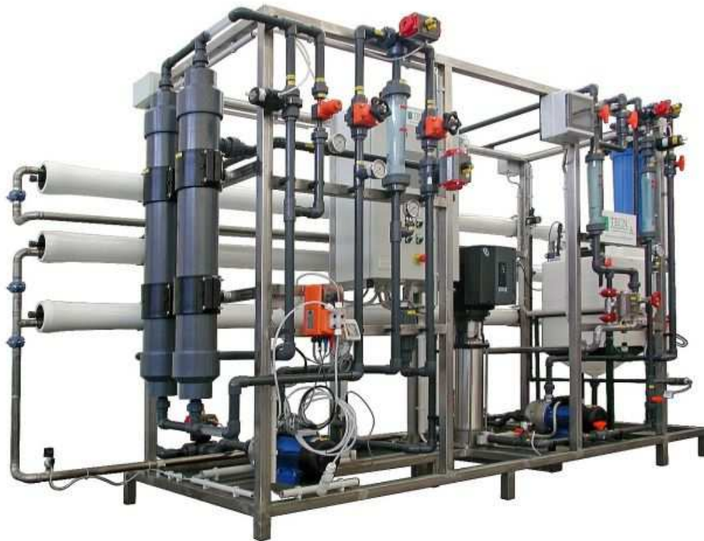
UF combined on RO skid
